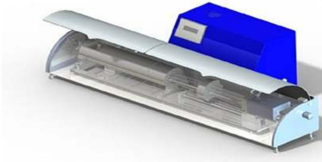
**Figure: Multi Thermal Gradient (MTG) freezing systems.**
